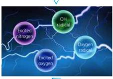
The electrons collide and combine with nitrogen and oxygen in the air to form four kinds of decomposing elements with decomposition power.
